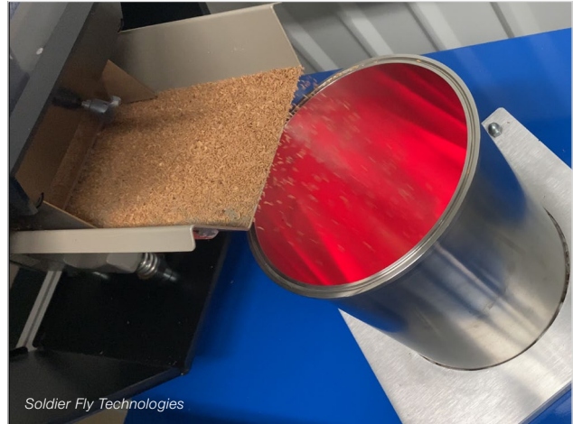
The Sciotech Counter counting BSF neonates (newly hatched larvae), providing the essential data for scientifically precise colony management
